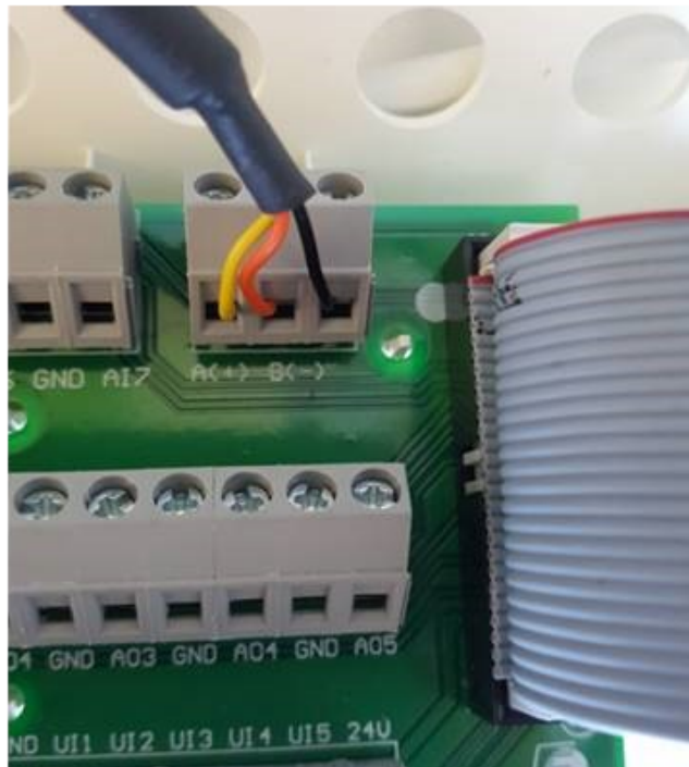
Fig. 1 Connection of the RS485 to USB on the connection box. GND connection not necessary
